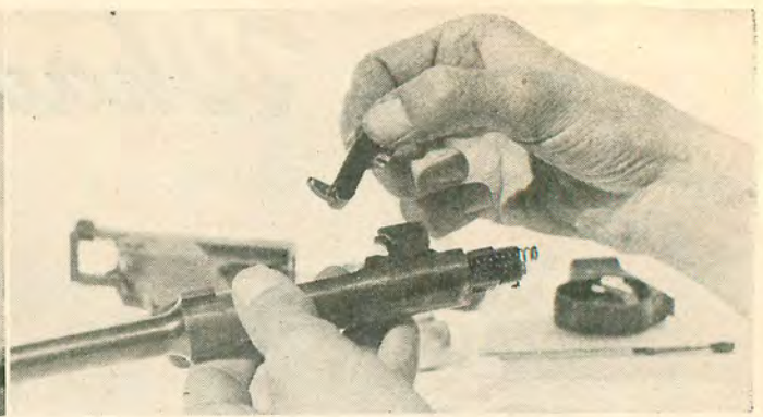
Lifting out the lock. The inner surfaces of the arm are well machined and finished
