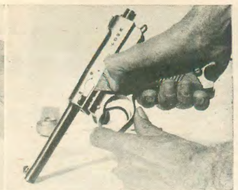
Removing trigger unit. Arrow shows safety is off in forward position
