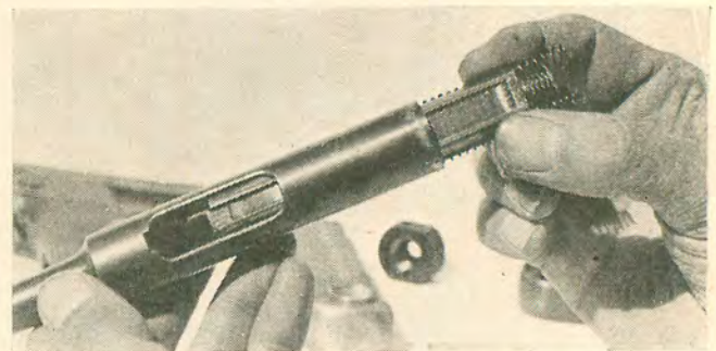
Above, removing bolt and return springs
